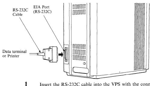
Insert the RS-232C cable into the VPS with the connector indicating the same direction.
