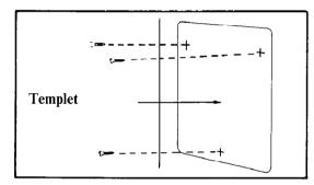
2 Install the 3 screws into the wall.
