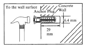
**3** Install the 3 screws into the anchor plugs.
